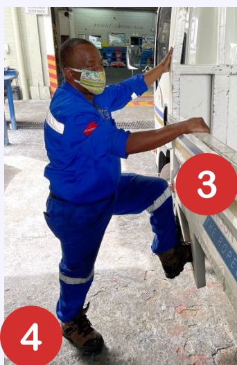
Figure 1: Three (3) point contact to be maintained when embarking or disembarking trays. To disembark
