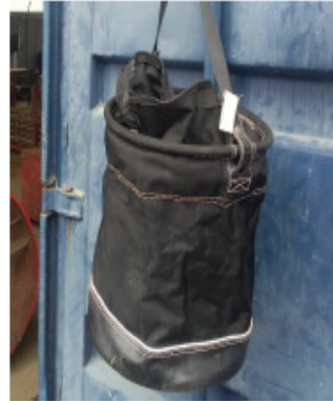
Figure 1: Clamp bags must be used for passing clamps during erection and dismantling of scaffolding. Ensure that the Working Load Limit is clearly marked on the bags.
