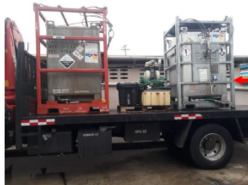
Figure 1: Example of a crash cage on top on the truck bed. Arrow shows height that the employee climbed to in order to straighten the straps.
